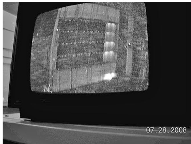
Figure 9.—Discharge on Teflon covered area at -2 kV bias voltage with beam energy at 2.8 keV and with a beam current density of 10 nA/cm 2 . Note: four lighted cells above arc site are due to reflections from the primary arc.
