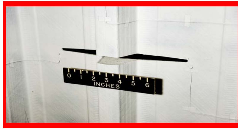
Figure 4. Notch in hat-stiffened panel.
