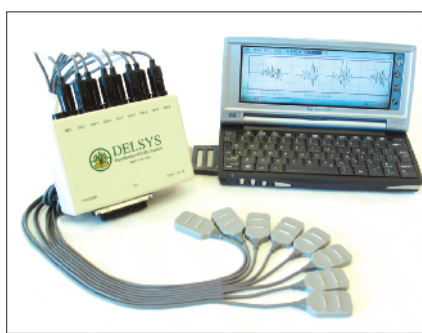
This Portable Electromyograph can record signals from as many as 16 differential EMG electrodes. The overall mass of the equipment is 1.1 kg. A wireless version of this device is scheduled for release in the near future.
