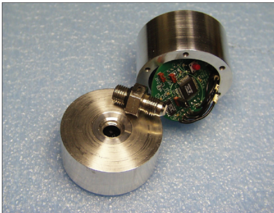
A Compact Unit Containing Eight Pressure Sensors, a microprocessor, and other circuitry generates not only a pressure reading of greater than usual precision, but also an assessment of its own reliability and remaining lifetime.
