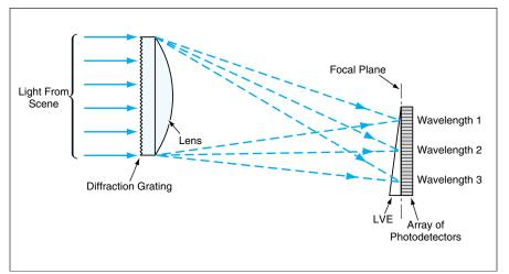
The LVE Would Be Matched, spatially and spectrally, to the focal-plane spectral dispersion pattern of the diffraction grating.
