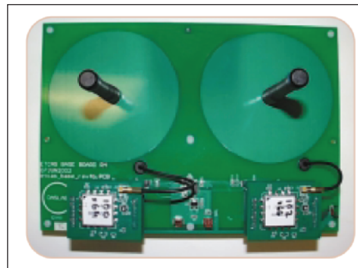
The Central Station Hardware includes communication modules that contain generic RF circuit boards. Identical communication modules are used in the remote stations.
