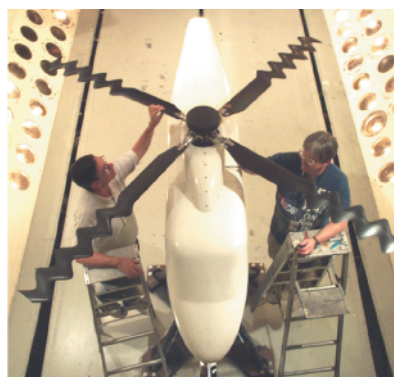
Wavy-Planform Rotor on Model Helicopter in Wind Tunnel
