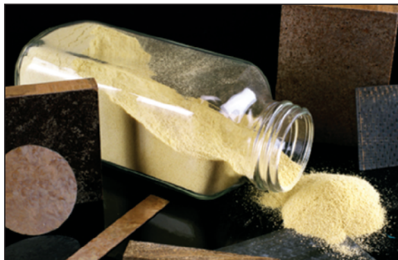
Several Products made from LaRC-LCR include films, plaques, foams, uniaxial carbon-fiber prepregs, and carbon-fiber composites.
