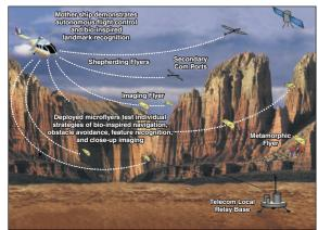
Figure 2: This is a **Conceptual Illustration of a Planned Demonstration**, "Bioinspired Engineering of Exploration Systems for MARS," to be performed at a MARS analog site on Earth. Here, microflyers work in synergy with the existing surface/aerial systems to enable new science endeavors. Multiple local comports provide a robust communication route for imagery downlink from the microflyers.
