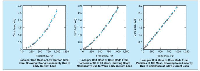
The **Total Losses as Functions of Frequency** were measured in three cores at a magnetic induction of 5 kilogauss (0.5 Tesla). In general, the total frequencydependent loss in a given core is the sum of a linear hysteresis contribution and a quadratic eddy-current contribution. Hence, the near-linearity of the curve in the 100-mesh case is evidence of low eddy-current loss.
