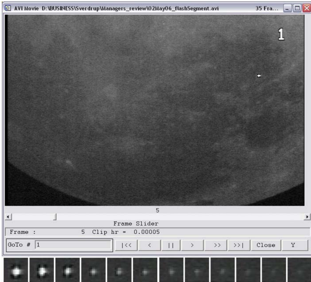
Figure 1. Lunar impact as seen on May 2, 2006 with a 254mm aperture telescope at 30 frames/second. The lower sequence shows a magnified view of the flash decay versus frame. This impact is one of the brighter impacts observed to date.
