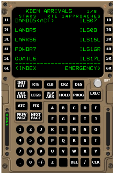
Figure 5: A CDU showing the Departures/Arrivals page for Denver (KDEN) airport. The emergency prompt appears next to button 6R at the lower right.
