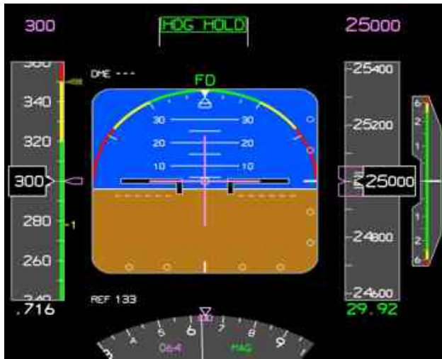
Figure 9: The Primary Flight Display (PFD) showing bank angle, pitch, airspeed, vertical speed, altitude and heading.
