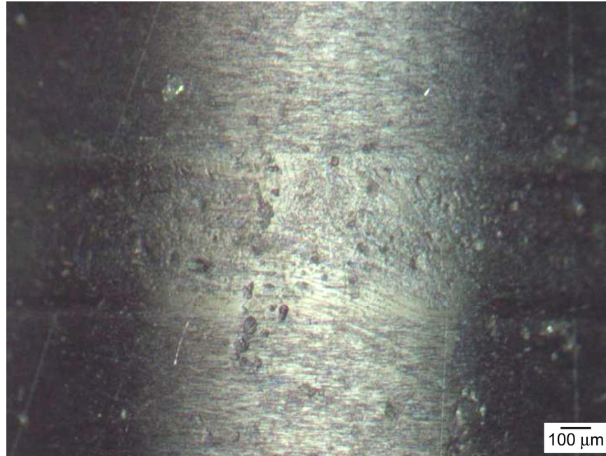
Figure 7.—Wear track surface following RCF test at 360 ksi, no failure observed.
