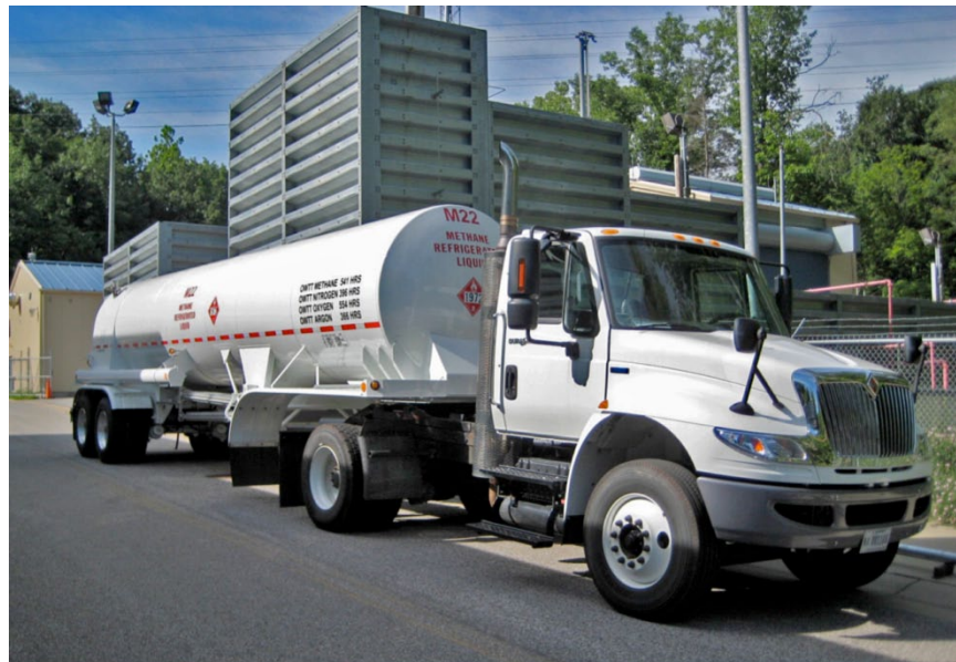
Figure 7.—15,100 liter liquid methane roadable Dewar (M-22).
