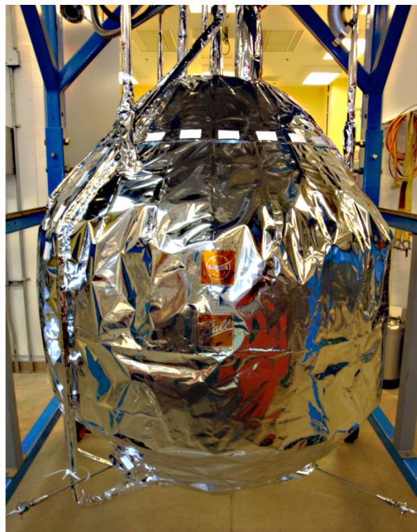
Figure 8.—Test tank covered in multilayer insulation (MLI).
