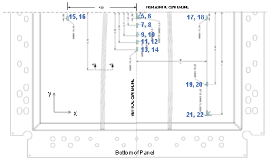
Figure A2. Location of strain gages on bottom half of test panel.
