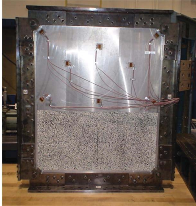
Figure 4. Picture frame support mounted on a generic test panel.
