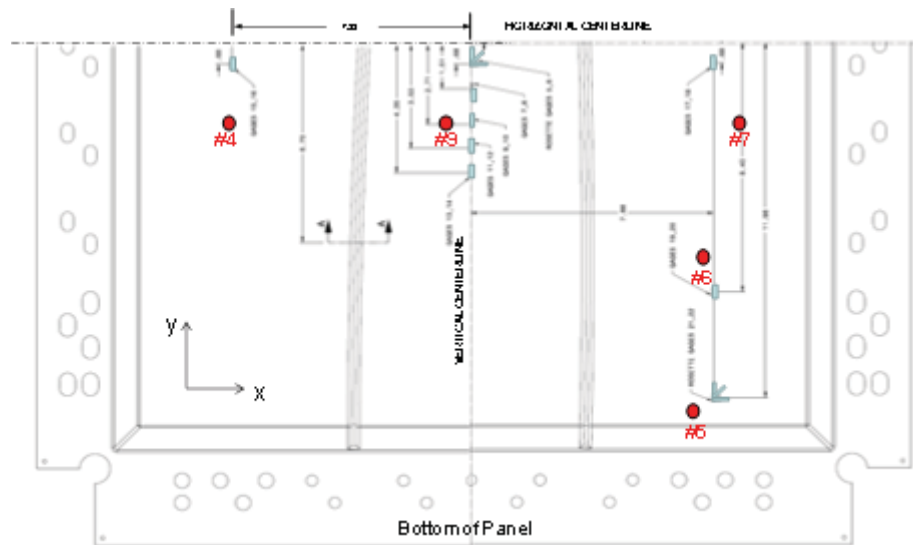
Figure B1. Location of LVDTs on test panel.
