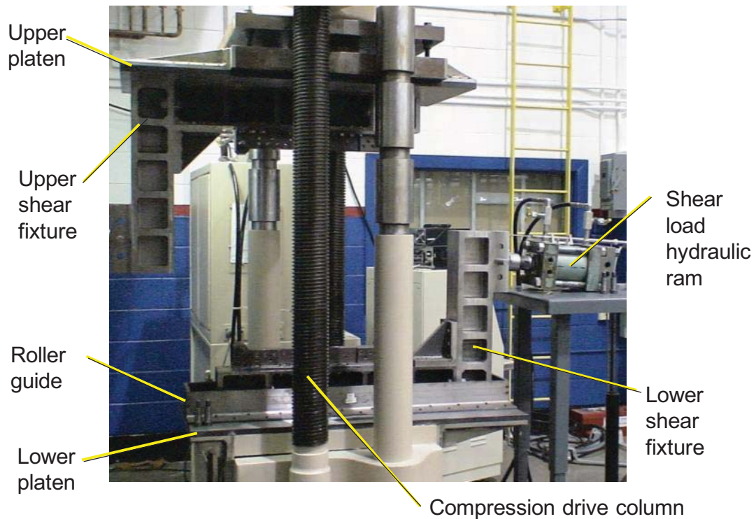
Figure 3. Compression-shear test system without test panel installed.
