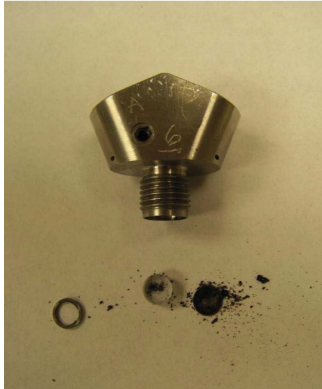
Figure 7.1-4. Sealing Ring, Sapphire Window, and Booster Charge Cover Simulator from the Modified SS V-Channel PCA
