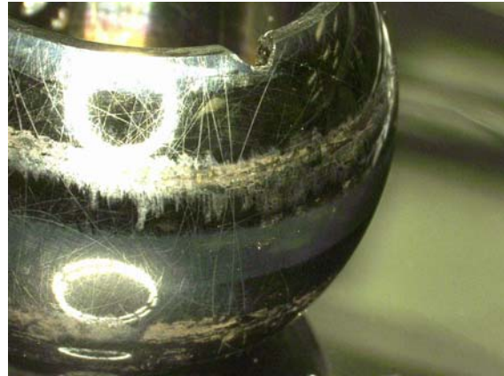
Figure 25: Spherical Ball after vibrate testing
