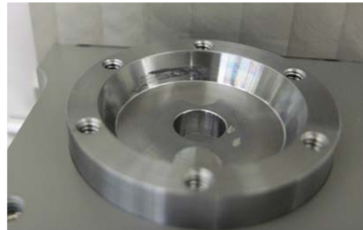
Figure 19: Lube wear on shear cup caused by fiber 180 degrees opposed
