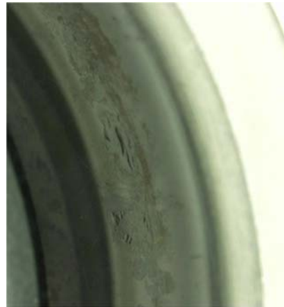
Figure 26: Spherical Bearing race wear
