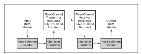
A **Unidirectional Serial Data Link** according to the proposal would be made from a commercial fiberchannel transmitter and receiver augmented externally with character translators and a Reed-Solomon encoder and decoder.
