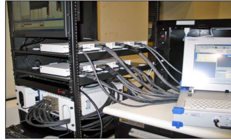
Fig. 20: Ares I US DFI MDAU, workstation, and sensors.
