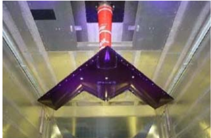
Figure 2. Stability And Control CONfiguration (SACCON). \Lambda_{le} = 53^\circ .
