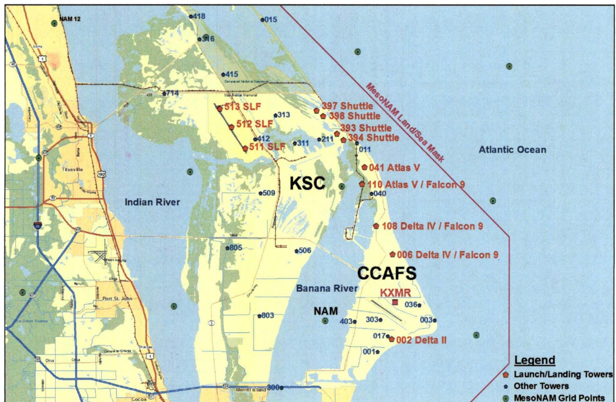
Figure 1. Map of KSC/CCAFS (from Bauman 2010) showing the locations of the wind towers used to verify MesoNAM forecasts (red pentagons labeled with tower number and the supported launch activity), the locations of the MesoNAM model grid points (green circles with black dot) and CCAFS weather station (magenta square labeled KXMR). The model grid point labeled “NAM” represents the point data used by the 45 WS. The MesoNAM land/sea mask is shown by the magenta line.
