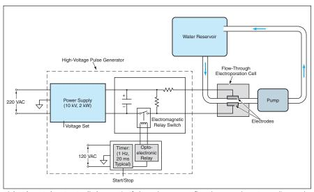
High-Voltage Pulses Are Applied to a pair of electrodes as water flows between them. Depending on the pulse amplitude, the resulting electric field between the electrodes either makes pathogens in the water more vulnerable to a disinfecting chemical or else inactivates them even in the absence of such a chemical.
