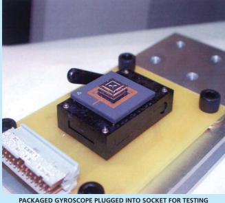
A **Plug-and-Test Design** enables the testing of many microgyroscopes in a short time.
