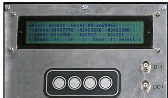
Figure 11. The SDA system LCD screen displays the results of real time inspection. The second row displays two resonant frequency locations, labeled #1 and #2. The four circular buttons are used to navigate through the screen as well as to perform various functions such as saving the signal response from the accelerometer.
