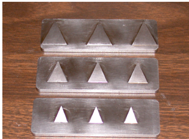
Figure 1. Picture of three micro-ramp inserts from the experiment in the 15 x 15 cm supersonic wind tunnel.
