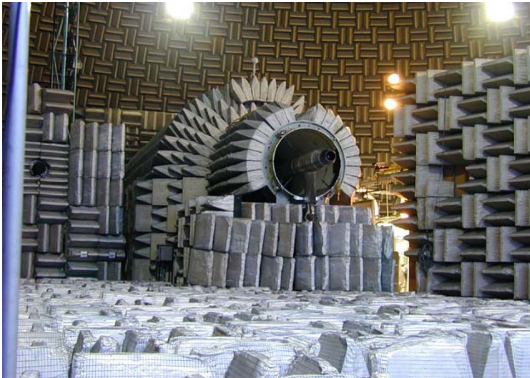
Figure 1: Nozzle Aeroacoustic Test Rig (NATR) inside the AeroAcoustic Propulsion Lab.
