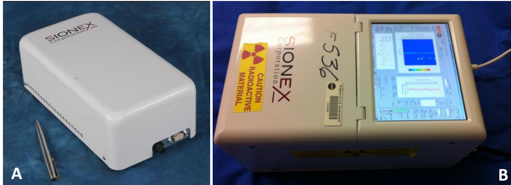
Fig 2. Air Quality Monitor, based on gas chromatography/differential mobility spectrometry. (A) Experimental version of the AQM which has operated on ISS since 2009. (B) Operational version under development to be delivered to ISS in early 2013. Dimensions are approximately 10x6x5 inches. The unit weighs 6.6 lbs. Each unit will have an estimated 2 year life.
