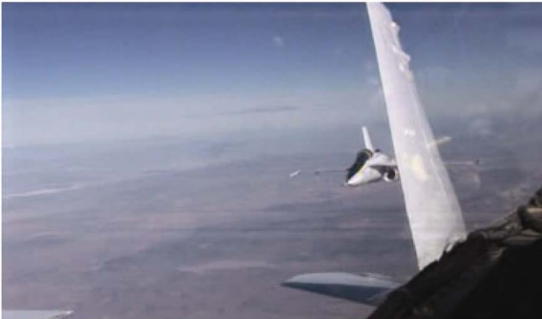
Figure 22. Lead aircraft view of the test aircraft during the fine tracking portion of the in-trail formation task.
