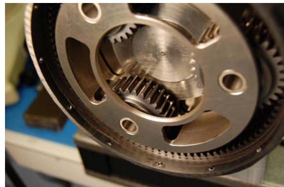
Figure 9. LTM0 gearbox during inspection after 30 million revs (at motor)
