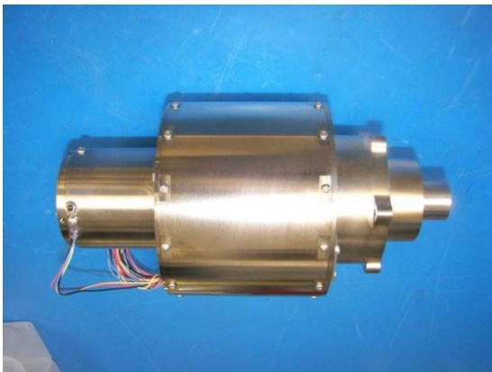
Figure 3. LTM1: 2 nd generation extreme environment actuator built by Aeroflex, Inc
