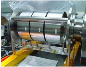
Figure 12. SMA main bearings Life Test setup and preloaded bearing capsules (3 pairs).
