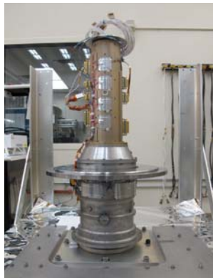
Figure 10. SMA mounted in test fixture to prepare for acceptance test in the clean room.
