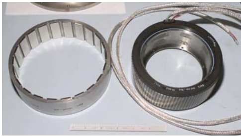
Figure 8. BAPTA (not GMI) 3-Phase DC torque motor.
