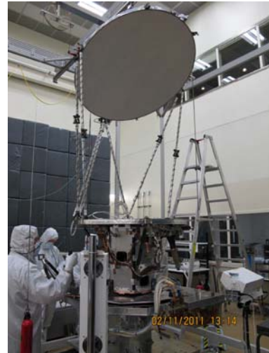
Figure 16. GMI Instrument during initial SMA Spin testing in Cleanroom with the reflector deployed
