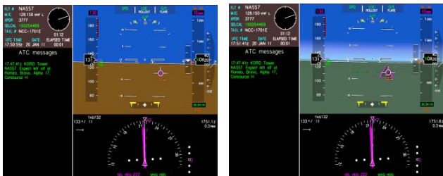
Figure 4. Baseline (left) and SVS (right) HDD Configurations
