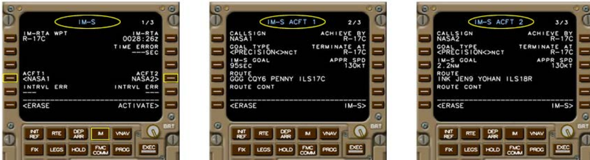
Figure 4. Three MCDU pages of ASTAR10 spacing tool displaying RTA plus IM clearance.
