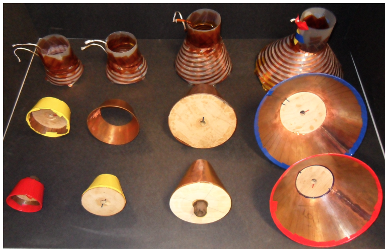
Figure 6. Coils and copper conic frusta used in the experiment.
