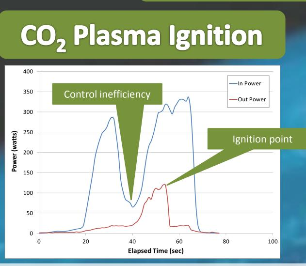
The sudden decrease in reflected power indicates when the plasma ignited in the PPA reactor. Note:  $CO_2$  ignition pressure = 30 torr, operating pressure = 45 torr
