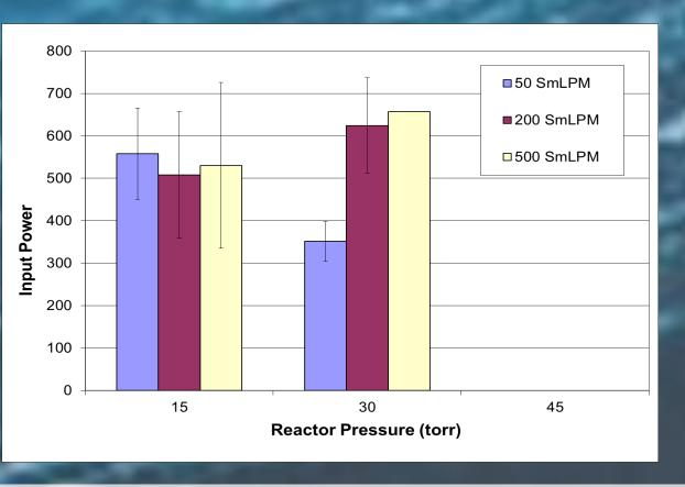
Testing indicated that CO<sub>2</sub> plasma was more easily ignited at lower pressures. It was not possible to ignite the  $CO_2$  plasma at 45 torr.
