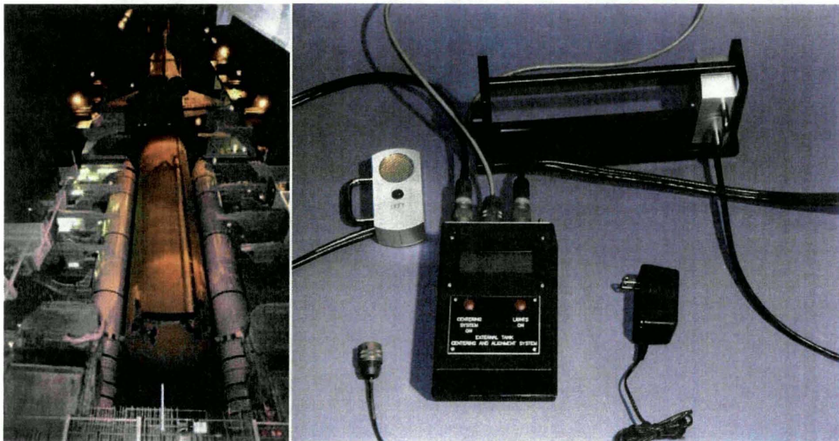
Figure 1. The External Tank Centering and Alignment System. The first major deliverable to the KSC Space Shuttle Program from the Applied Physics Lab was a system that measured the gaps between the Solid Rocket Boosters and the External Tank at the aft end.
