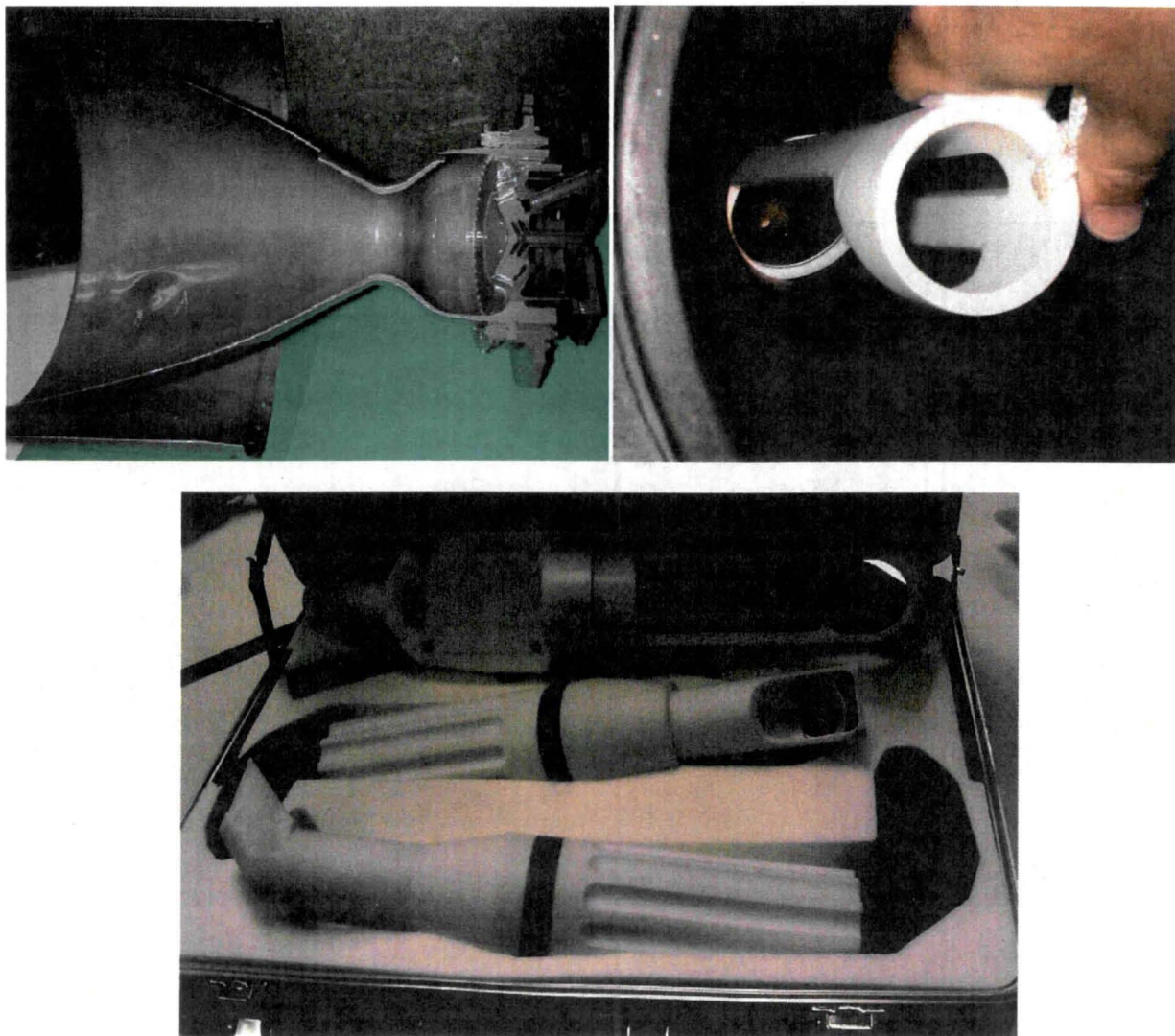
Figure 8. The RCS Nozzle Inspection Tools. The upper left image shows a cut away cross section of a Reaction Control System (RCS) Thruster. Thrusters, such as this, allow the Orbiter's position and orientation to be controlled while in orbit. Tools were designed and constructed, shown in the lower image, to allow these to be inspected. In the upper right one of these tools is shown imaging a small defect on the inner surface of the nozzle within the reaction chamber.
