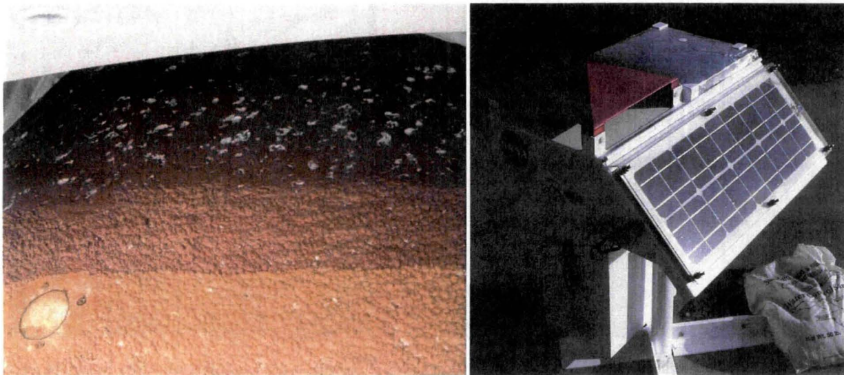
Figure 18. A HailStone Monitoring System. On the left side is an image of hail induced damage on the External Tank foam. On the right hand side is a hail monitor developed by the KSC Applied Physics Laboratory and used to support Shuttle launches.
