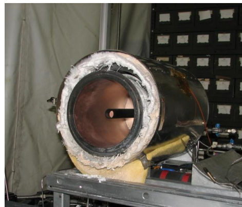
Figure 1. Open H-Bosch reactor.
