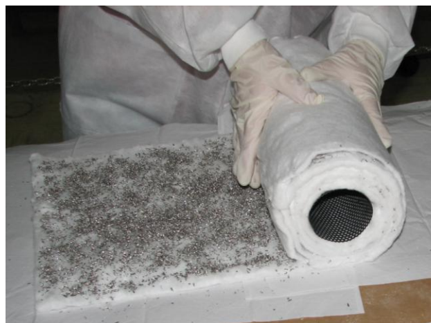
Figure 3. Layers of Co-Sh on insulation being placed around cartridge center.
