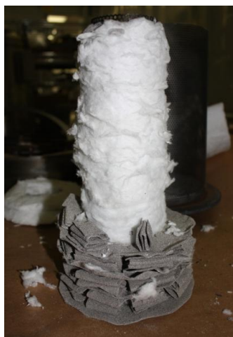
Figure 2. Center mesh piece from catalyst cartridge with part of NiF packing.
