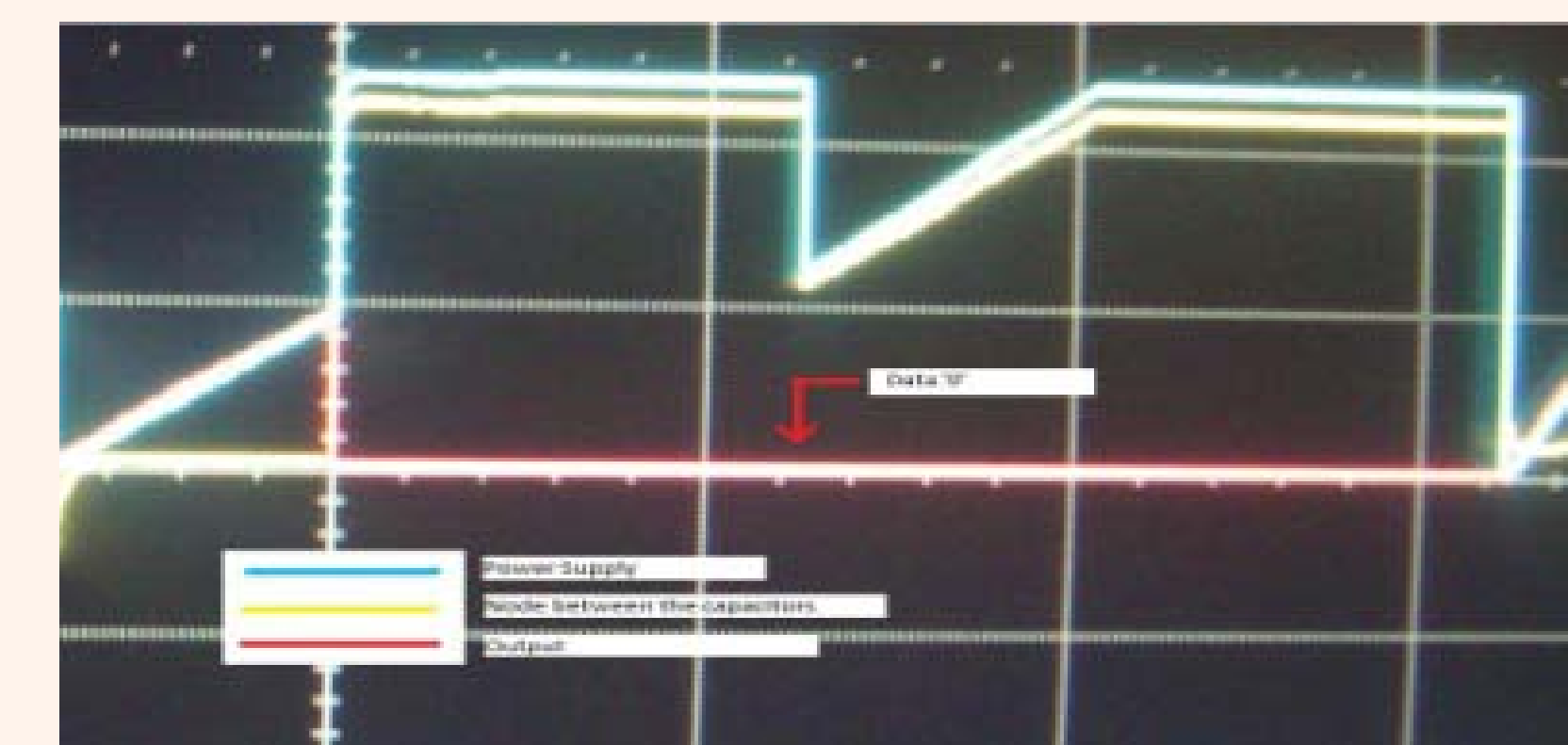
Figure 5: Reading a '0' from the latch
