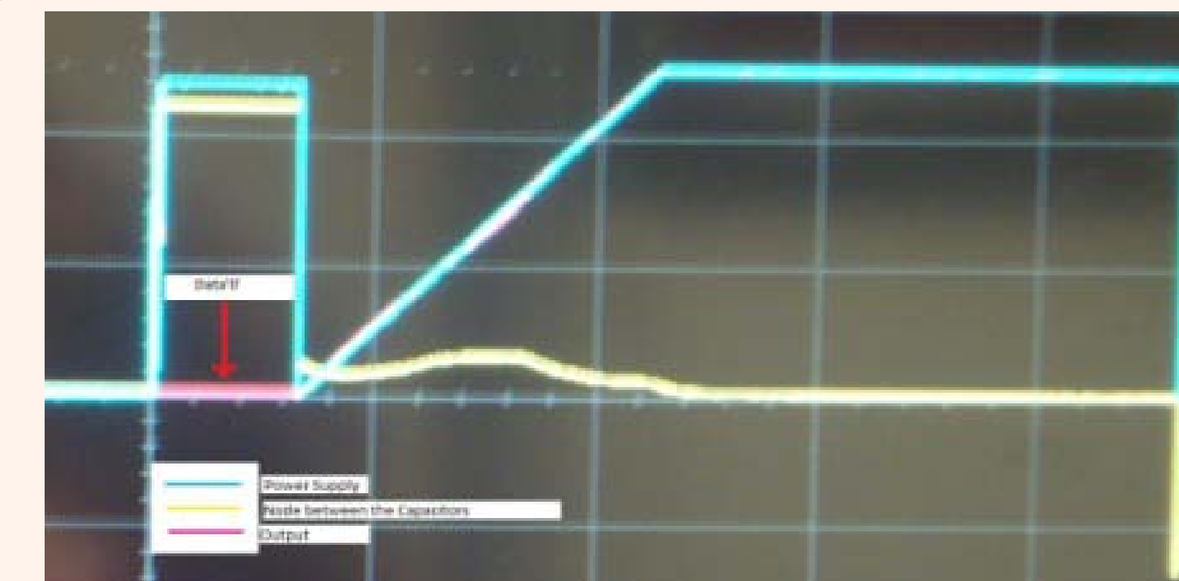
Figure 3: Writing a '0' to the latch
