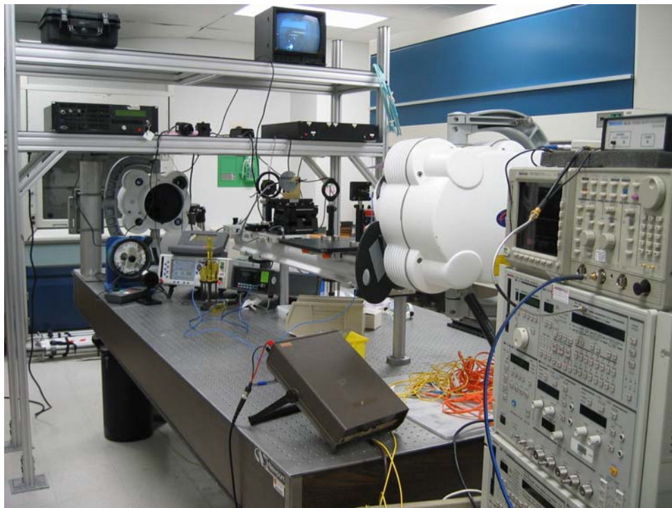
Figure 2-4 fSONA Units Being Tested In The SpaceHab Optical Lab
