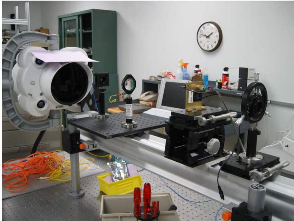
Figure 2-5 Beam Measurements Between OTU #1 & OTU #2
