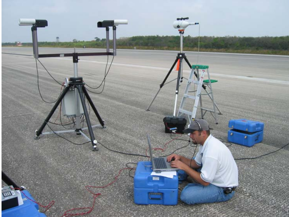
Figure 2-25 Wx Station and Scintillometer Rx on SLF
