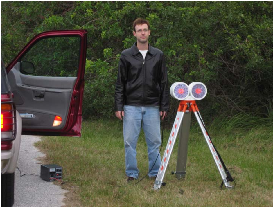
Figure 2-26 Transmit Portion of Scintec Scintillometer
