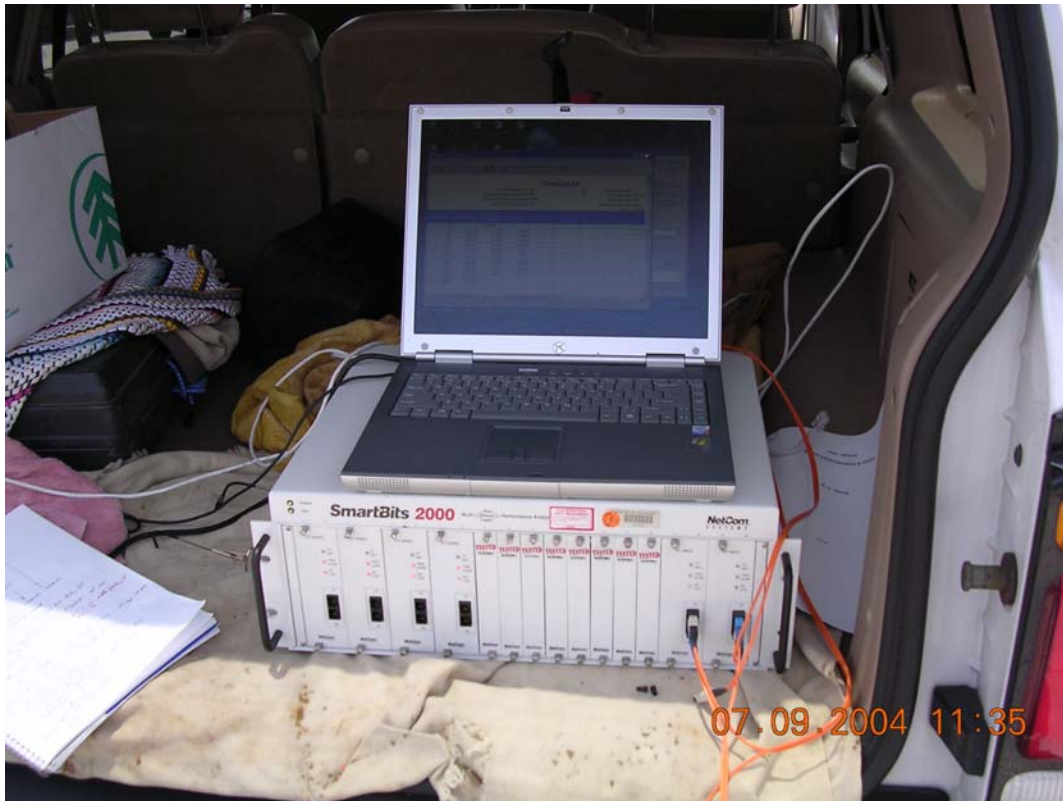
Figure 2-24 Field Testing with the SmartBits & a Laptop
