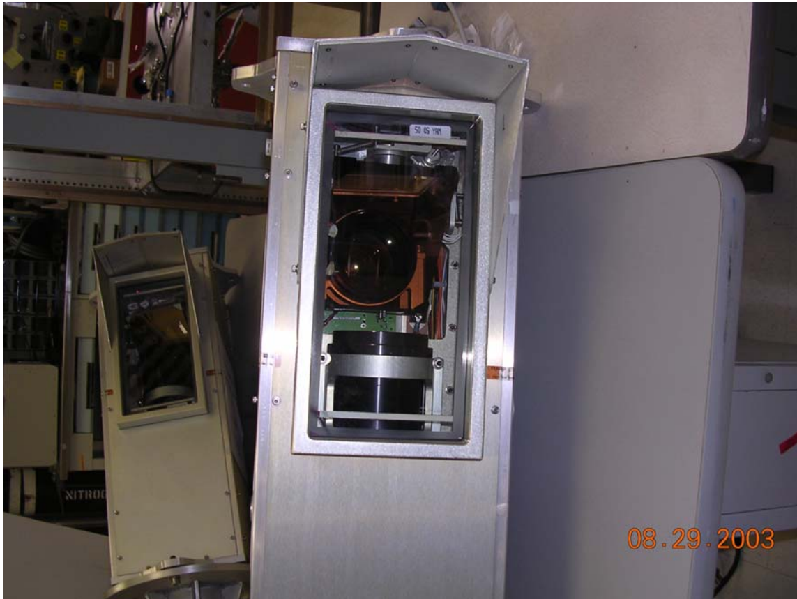
Figure 2-23 AirFiber 5800 With Fiberglass Shroud Removed
