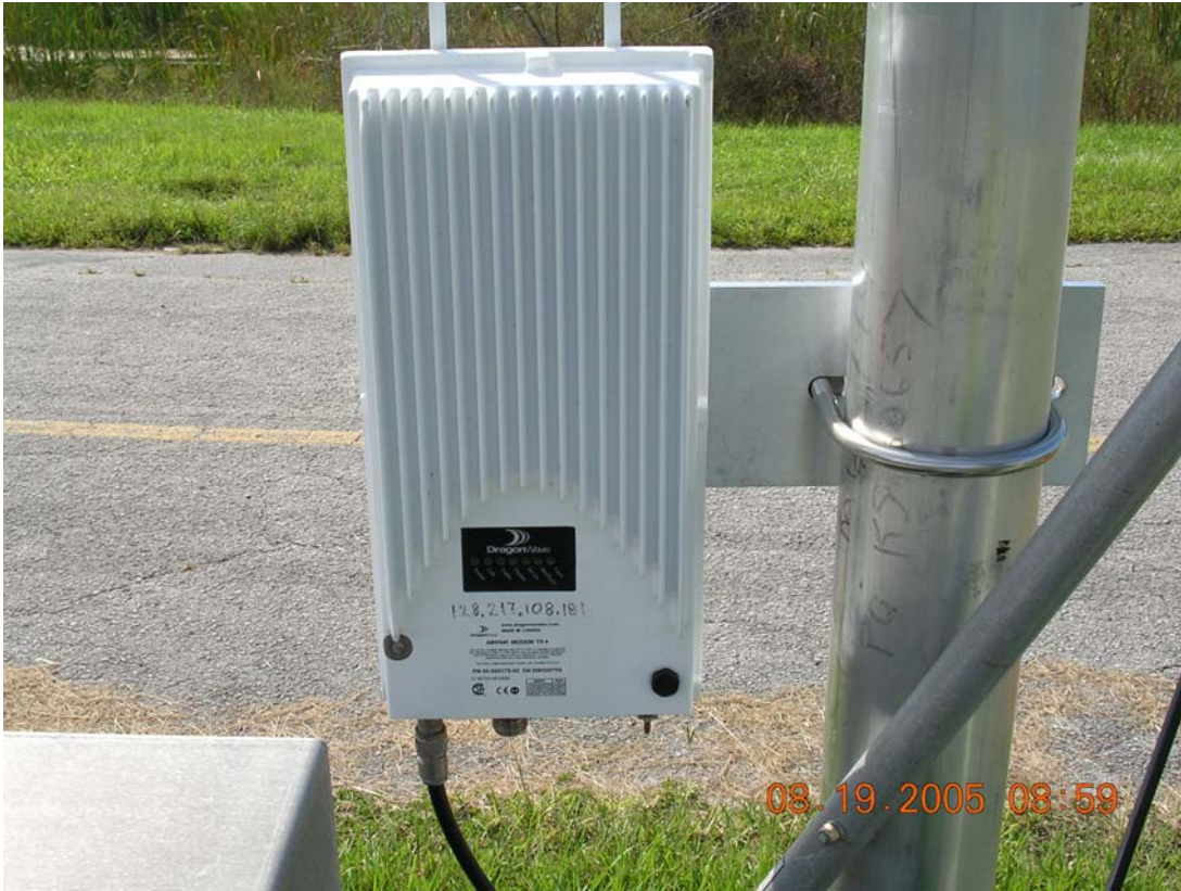
Figure 3-4 AirPair 100 Outdoor Modem
