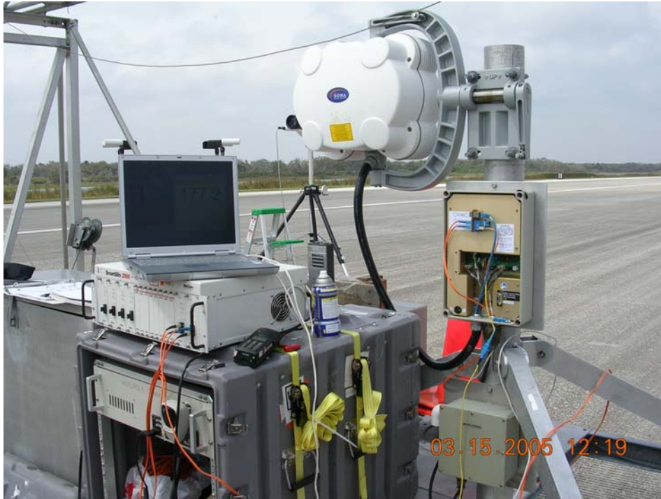
Figure 2-15 fSONA #1 With SmartBits, Laptop & Open Control Panel
