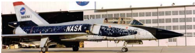
Figure 2: NASA F-106 aircraft with lightning attachment locations marked. 10
