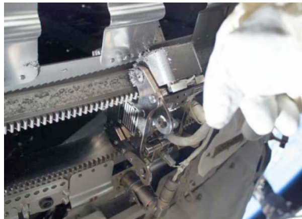
Figure 8.—Starboard SARJ on orbit after approximately 3 months of operation. Contacting race-roller surfaces are highly damaged.
