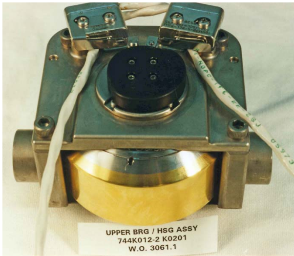
Figure 10.—Port SARJ upper roller showing intact gold plating prior to assembly into trundle.
