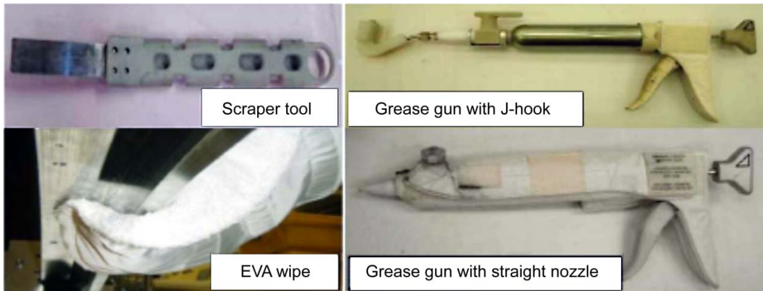
Figure 19.—Tools used in SARJ repair and recovery through cleaning and lubrication (from Ref. 5).
