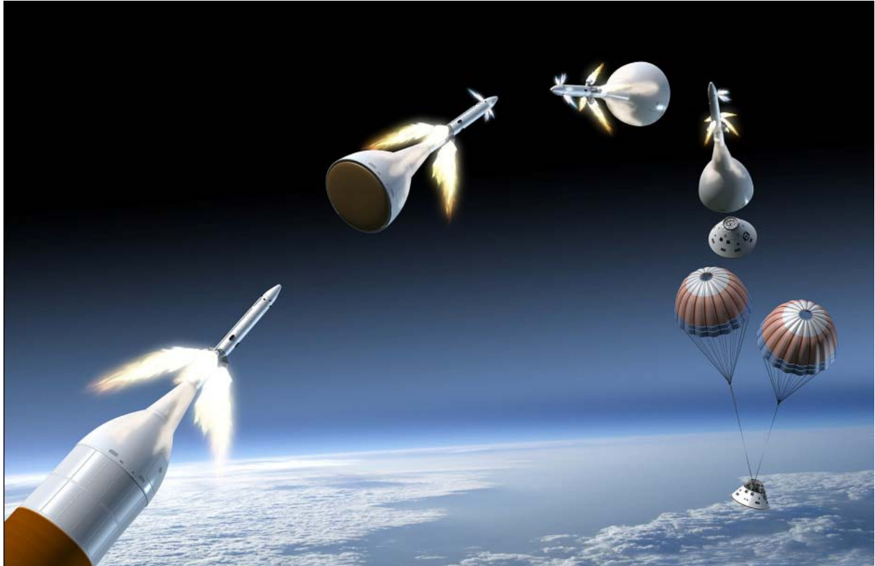
Figure 2. Illustration of the concept of operations for an abort from the launch vehicle.
