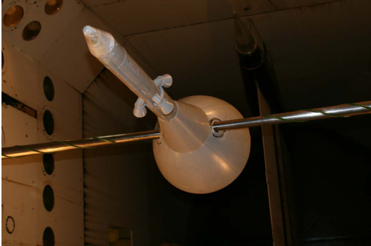
Figure 9. Orion 11%-scale ALAS Launch Abort Vehicle mounted to the traverse sting for forced oscillation and free-to-oscillate testing in the NASA LaRC Transonic Dynamics Tunnel.
