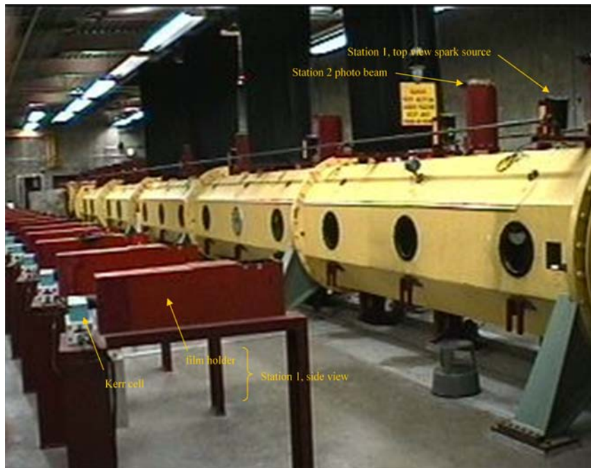
Figure 13. NASA-ARC Hypervelocity Free-Flight Aerodynamics Facility (HFFAF) test section
