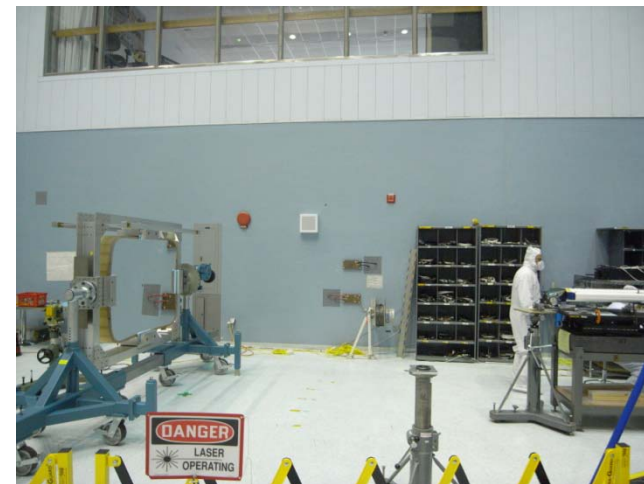
JWST GSE mirror and interferometer (SSDIF clean room, NASA GSFC)
