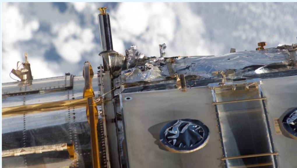
On-orbit insulation degradation and embrittlement
