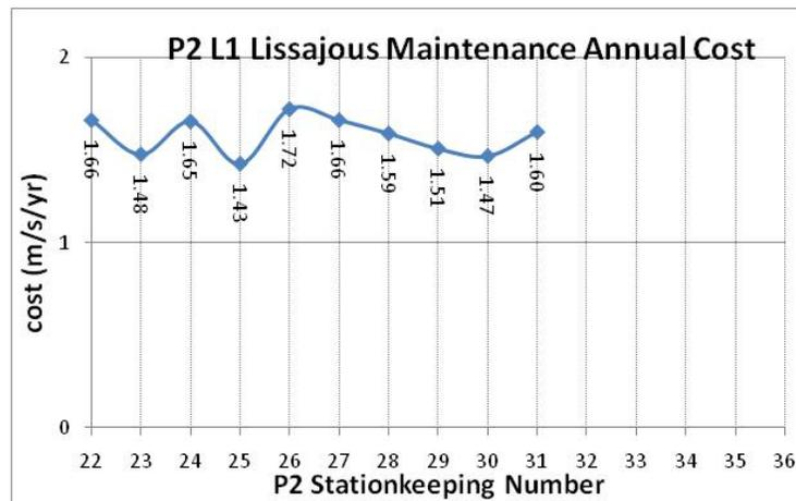
Figure 11. P2 EM L<sub>1</sub> Lissajous Orbit Cumulative Annual  $\Delta v$  Cost (Post Cr change)
