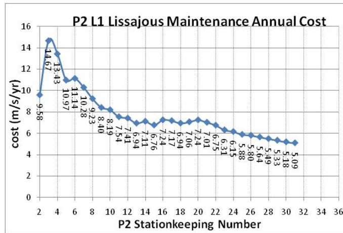
Figure 10. P2 EM L<sub>1</sub> Lissajous Orbit Cumulative Annual  $\Delta v$  Cost (Pre Cr change)
