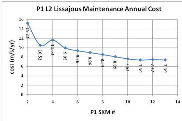
Figure 7. P1 EM L<sub>2</sub> Lissajous Orbit Cumulative Annual  $\Delta v$  Cost
