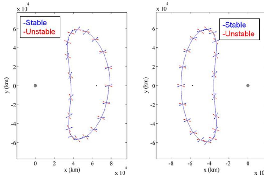
Figure 12. P1 EM L<sub>2</sub> and EM L<sub>1</sub> Stable and Unstable Directions
