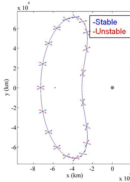
Figure 14. P2 EM  $L_1$  Stable and Unstable Directions
