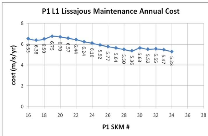
Figure 8. P1 EM L<sub>1</sub> Lissajous Orbit Cumulative Annual  $\Delta v$  Cost
