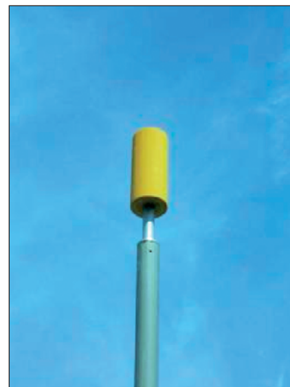
Figure 2. A Cylindrical Windscreen Covers a Microphone mounted on a pole outdoors.
