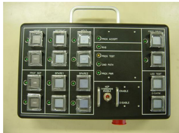
Figure 11, HTV Control Panel (HCP)
