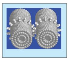
Two Molecular-Scale Gears are shown meshing in this computer-simulation image. The gears would include multiwalled carbon-nanotube shafts, to which gear teeth in the form of benzvne molecules would be bonded.
