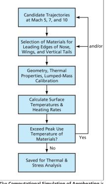
The Computational Simulation of Aeroheating is one of several real-time simulations used in initial design studies. This simulation can be used to eliminate flight trajectories that would give rise to local temperatures in excess of structural-design temperature limits.
