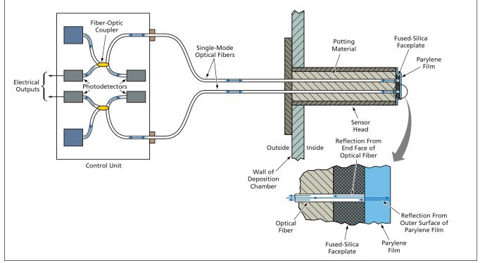
Portions of the Light Beam in each optical fiber would be reflected from opposite faces of the parylene and would interfere in one of the photodetectors. Variations in the photodetector output would be interpreted in terms of increases in the thickness of the parylene film according to well-known principles of interferometry
