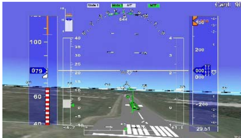
Figure 4. Offset landing as seen on the research pilot Heads Up Display.
