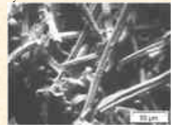
Ames Low density PICA: density = 0.229 g/cm 3 Thermal Diffusivity = 0.929 mm 2 /s Thermal Conductivity = 0.188 W/mK
